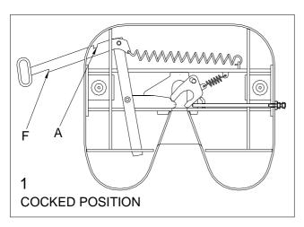
1. Before coupling, the Q Coupler is pre-set by lifting up and pulling out the operation handle 'F'. Secure handle notch 'A' on coupler plate (or in cocked position shown in figure 1).
